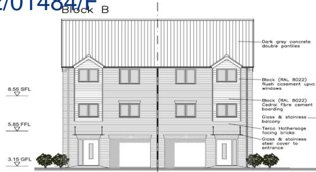
Front East Elevation
